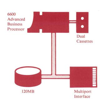
The 4650 DATASHARE system includes 6600 processor, 120MB of disk storage with controller, 9462 Multiport Interface, dual cassettes, and system software.
