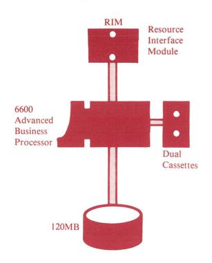
The 4654 ARC File Processor system includes 6600 processor, dual cassettes, 9483 Resource Interface Module, 120MB of disk storage with controller, and system software.
